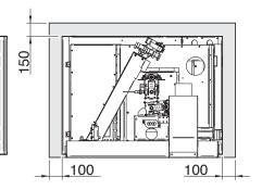
Furthermore, it is necessary to firmly fix the base of Inserto Paris to the support surface, using the most suitable system for the material this surface is made of. Anchoring the base is important to extract Inserto Paris safely.
