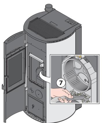
Unburnt residue inside the crucible can be vacuumed but can also be made to fall onto the bottom with a scraper, from where they will then go into the ash collection drawer. Once cleaning is complete, the burner lid can be refitted and closed, carrying out the same operations in reverse order.
