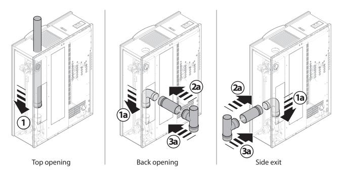
Inserto Paris is supplied from the factory with an arrangement for bayonet connection to the flue (upper smoke outlet only).
