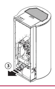
Rotate the fume motor for the side outlet according to the stove model, unscrewing the 2 screws (4).
