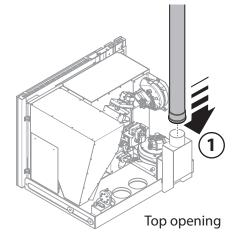
Inserto Paris is equipped with a slide that allows it to be pulled out halfway through the depth. By unscrewing the two lateral screws it is possible to extract it completely.
