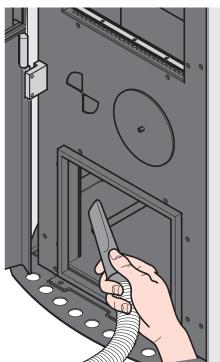
In the Inserto Paris model, cleaning must be done on the inspection drawer by unscrewing the appropriate screws.
